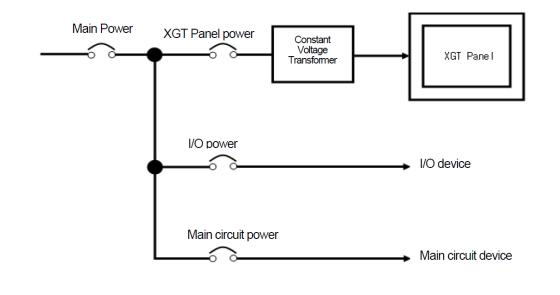
Separate the XGT Panel power from the I/O device and main circuit device.
