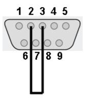
The RS-485 and RS-422/485 port terminal should be made as follows. (Only eXP2-07xx/10xx)
